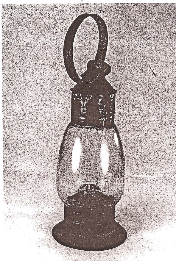
Figure 3.19 - (Upper left) This star-diamond-star pattern, fixed globe lantern (SDS-4) has a tinned steel frame with a japanned finish. The globe is cast "BC&MRR" (Boston, Concord and Montreal Railroad).
